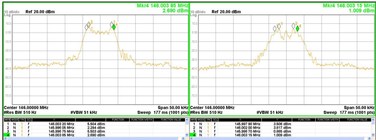
Figure 16: FM spectra of a 400Hz (left) and 1kHz (right) tone at 400mV p-p
